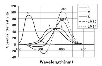
Figure 4. New red sensitive distribution given by linear combination of LMS functions
