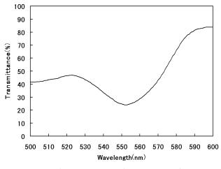
Figure 3. Transmittance of green sensitive layers
